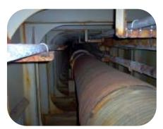
Ballast pipe on a 300mtr grain carrier had become so badly corroded the vessel was struggling to take on board ballast. Due to the confined space and restricted access the surfaces of the pipe could only be manually abraded. Once cleaned 302 Epoxy Repair Cement was applied to the repair surface. 301 Epoxy Resin and Hardener and Glass tape were applied once the repair paste had cured
